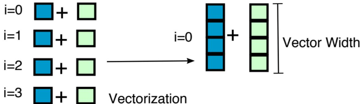
The addition operation is applied to all the data from  $i = 0$  to  $i = 3$  *at the same time*.
