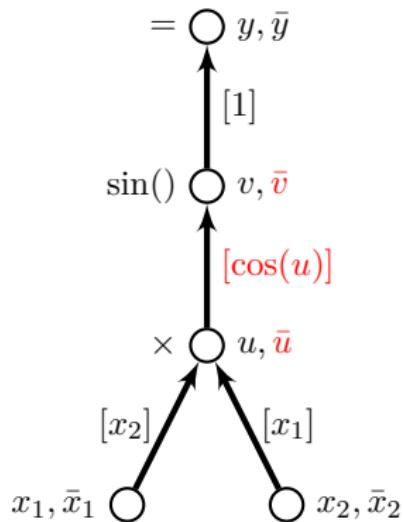
$$\bar{x} = \bar{y} \cdot F'(x) = \bar{y} \cdot \frac{\partial y}{\partial x} = \underbrace{\bar{v} \cdot \frac{\partial v}{\partial u}}_{=\bar{u}} \cdot \frac{\partial u}{\partial x}$$
