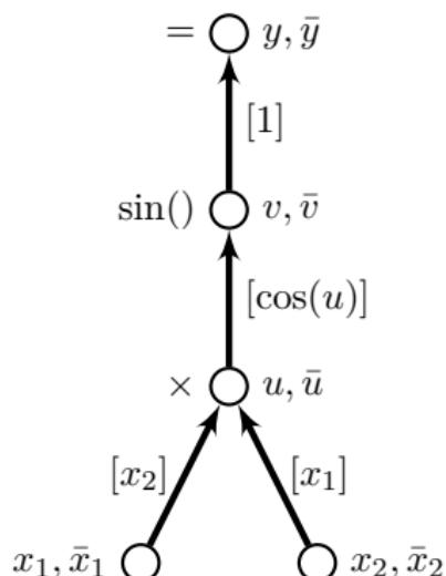
The control flow of the program must be reversed, intermediate results are required for the reverse sweep!
