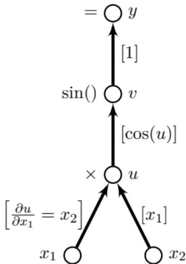
$$\bar{x} = \bar{y} \cdot F'(x) = \bar{y} \cdot \frac{\partial y}{\partial x} = \bar{y} \cdot \frac{\partial y}{\partial v} \cdot \frac{\partial v}{\partial u} \cdot \frac{\partial u}{\partial x}$$
