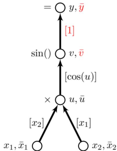
$$\bar{x} = \bar{y} \cdot F'(x) = \bar{y} \cdot \frac{\partial y}{\partial x} = \underbrace{\bar{y} \cdot \frac{\partial y}{\partial v}}_{= \bar{v}} \cdot \frac{\partial v}{\partial u} \cdot \frac{\partial u}{\partial x}$$
