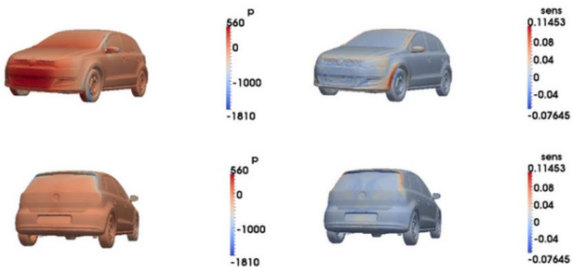
The figure shows **sensitivities of the drag coefficient** to each point on a car's surface when it moves at high speed (left) and low speed (right). The simulation was performed with **AD-enabled OpenFOAM** built on top of **dco/c++**. The normal simulation took **44s**, while the AD-enabled simulation took **273s**, to obtain the same gradient by finite differences would take roughly **5 years** (surface mesh had 5.5 million cells).
