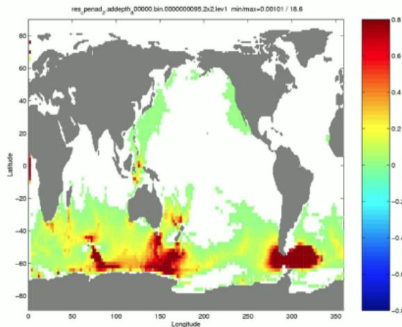
Obtaining the gradient through finite differences took a month and a half. The adjoint AD code obtained the gradient in less than 10 minutes.
